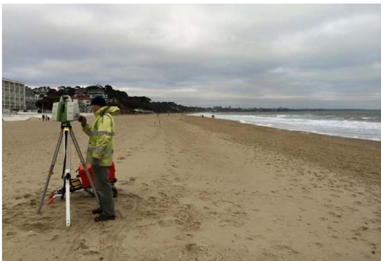
Figure 5: Leica C10 laser scanner on site
